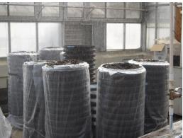
Figure 33. Columns under rainfall simulator.
