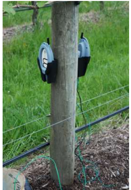
Figure 3: The Carta sense soil moisture and temperature monitoring device
