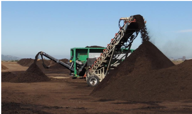
Figure 19. Compost screening at a municipal yard trimmings composting facility. Photo by Doug Pinkerton, courtesy of BioCycle.
