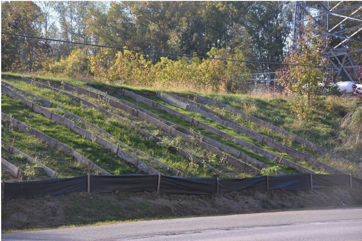
Figure 13. Erosion control study in Upper Marlboro, MD that compare the effects of compost blankets composed of various biosolids and yard waste compost mixtures on grass cover and sediment retention on steep slopes. Photo by Dylan Owen. Research sponsored by Maryland Department of Transportation - State Highway Administration.
