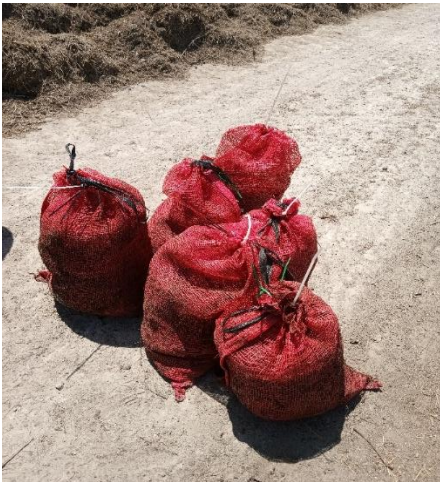
Compostable products from Eco-Products and BsiBio placed in the mesh bags and ready to be placed into the windrow.
